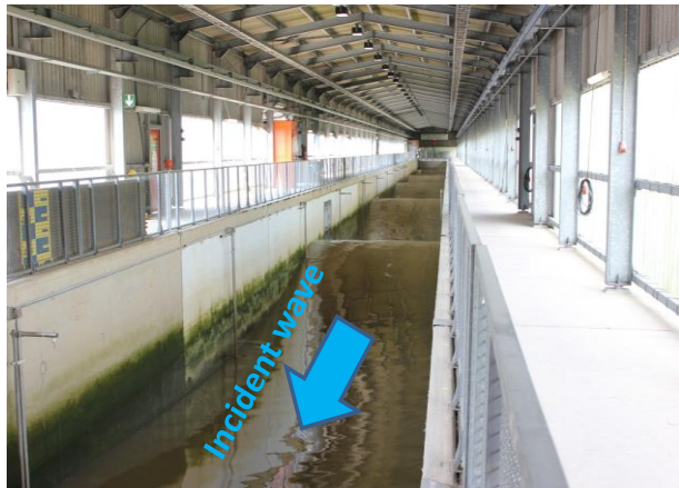
a) wave generation in the large scale wave flume
