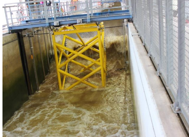
b) Incident wave approaching the truss structure
