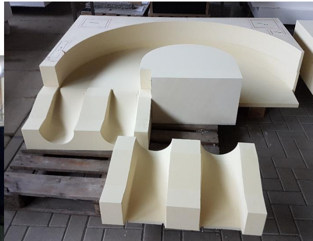
Inlet geometry made by milling from a massive block of polyurethane foam
