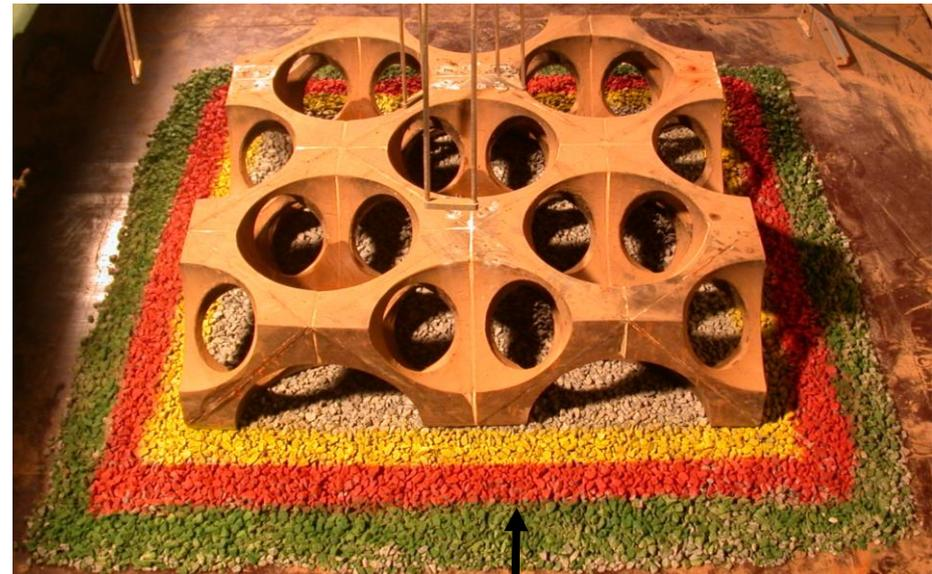
crushed gravel  $D_{50} = 0.0052 \text{ m}$
