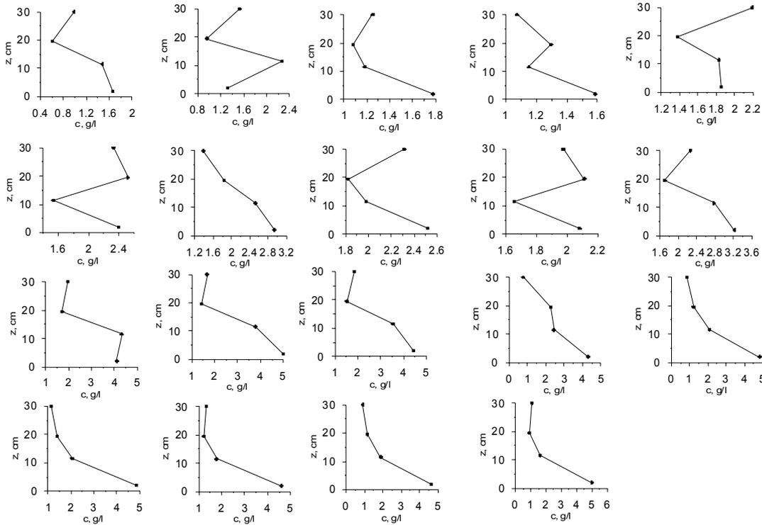
Fig. 4. High-frequency fluctuations of vertical profiles of suspended sediment concentration, each analyzed for a one second time segment from the time histories.
