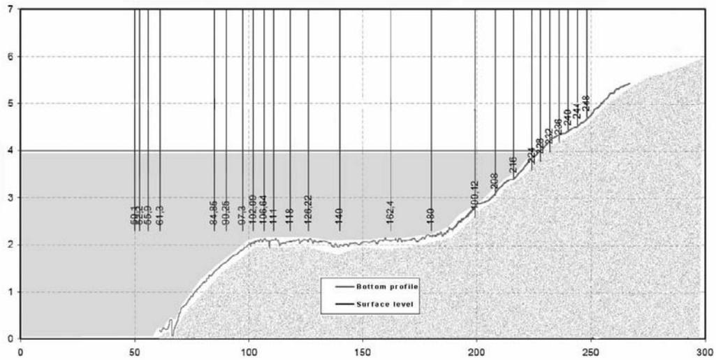
Fig.1. Longitudinal section of GWK with installed sand bed and wave gauges
