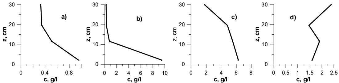
Fig. 5. Characteristic types of vertical distributions of suspended sediment concentration.
