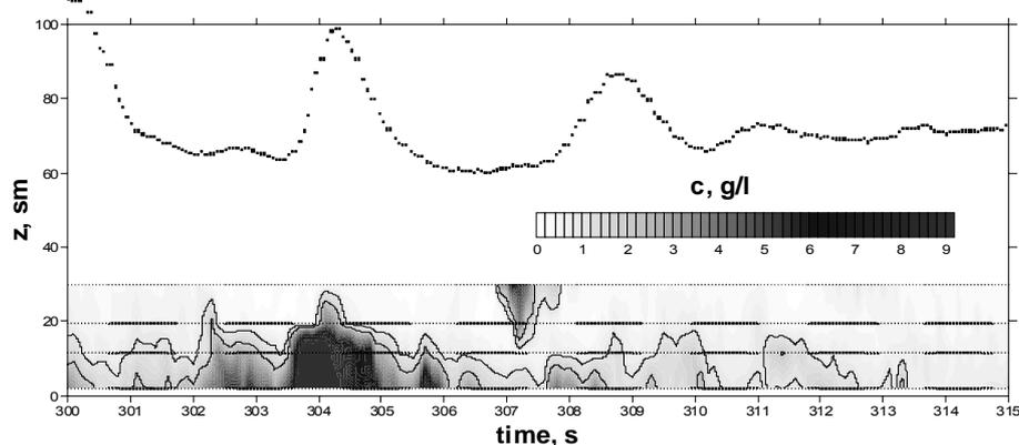
Fig.6. Chronogram of temporal fluctuations of the field of suspended sediment concentration and surface elevation
