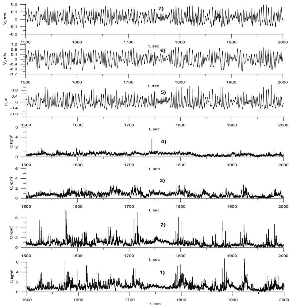
Fig. 3. Fragments of the recorded suspended sediment concentration fluctuations (turbidimeters 1-4 from 7, 15, 25, 40 cm above sea bottom), the synchronous free surface elevation  $H$  (5) and the water velocities from the Vector sensor, where  $v_x$  is the cross-shore (6) and  $v_y$  the vertical component (7) of velocity.
