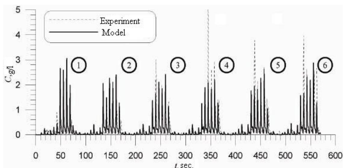
Fig.7. Comparison of concentration chronograms calculated on the model with those measured at 5.5 cm above sea bottom
