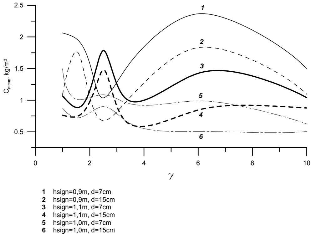
Fig. 8. Dependence of time averaged concentrations at two horizons (7 and 15 cm from sea bottom) for three significant waves heights ( $H_{sig} = 0.9, 1.0$  and  $1.1$ m) on spectral steepness.
