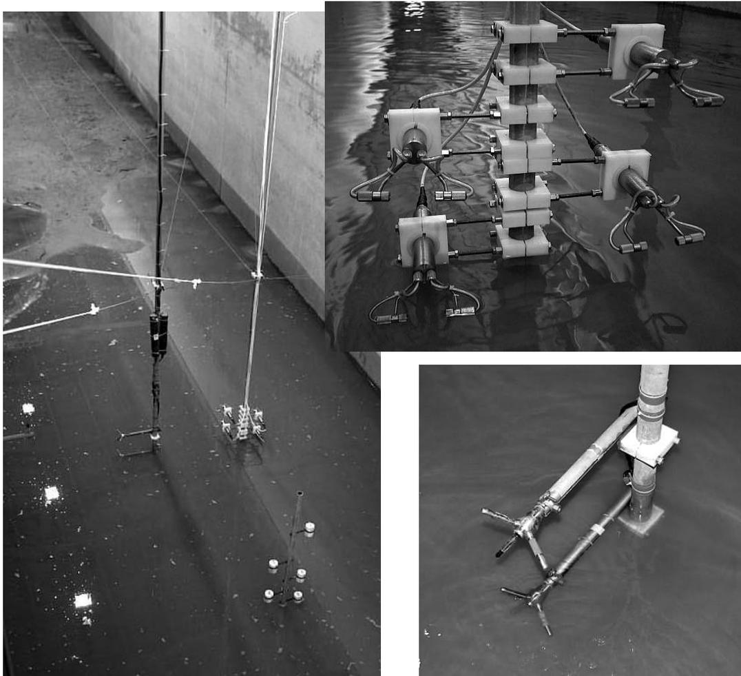
Fig. 2. Installed turbidimeters, velocity sensors (Nortek-Vector) and sediment accumulators (left hand photo). Positioning of turbidimeters (upper right photo) and velocity sensors (Nortek-Vector) (lower right photo)
