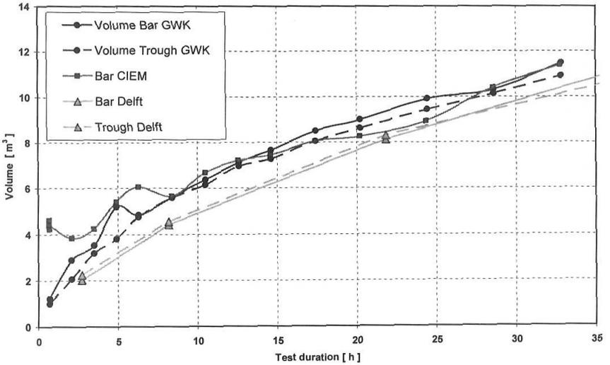
Figure 5. Bar and trough sand volume evolution along the time experiment.
