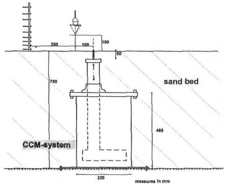
a) **Figure 7** a) Top view of the CCM tank (University of Twente) with the three electro-resistance probes for granular flow measurements and b) schematic plot of the tank set-up in the flume.
