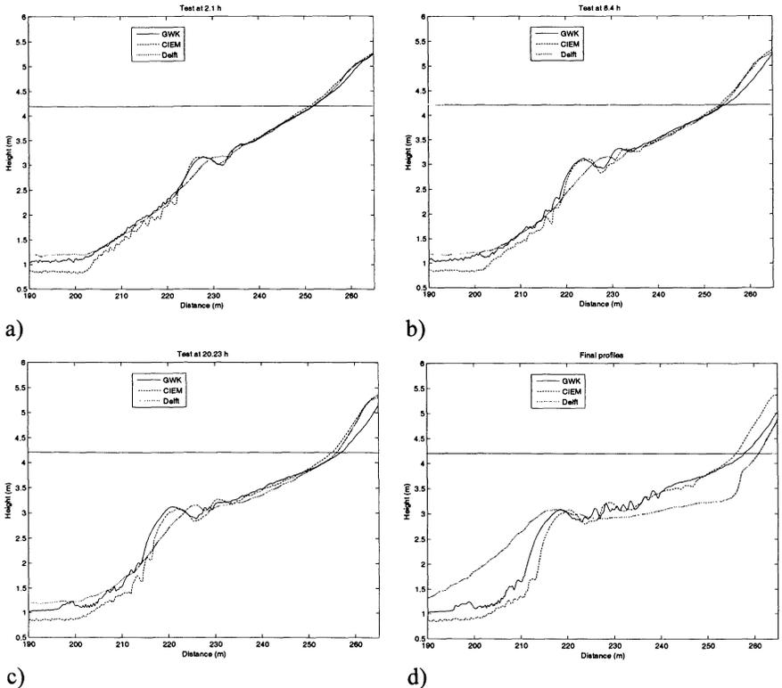
**Figure 3. Bed profile evolution in the three flumes under Erosive wave conditions.**
