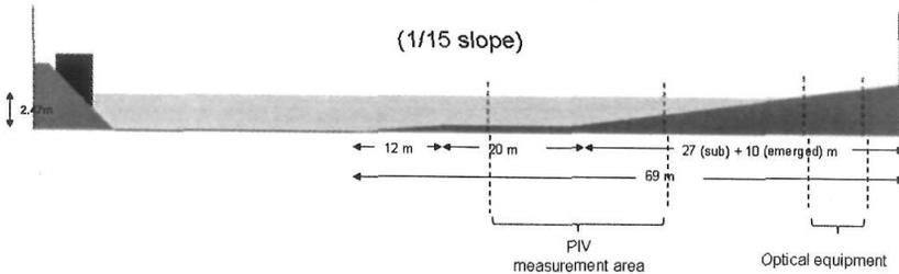
**Figure 2. Flume layout for the Barcelona CIEM experiments at scale 1/1.9 related to prototype (Hannover).**
