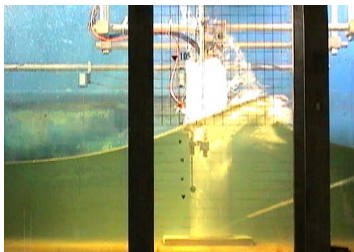
Figure 4. Breaking wave on cylinder
