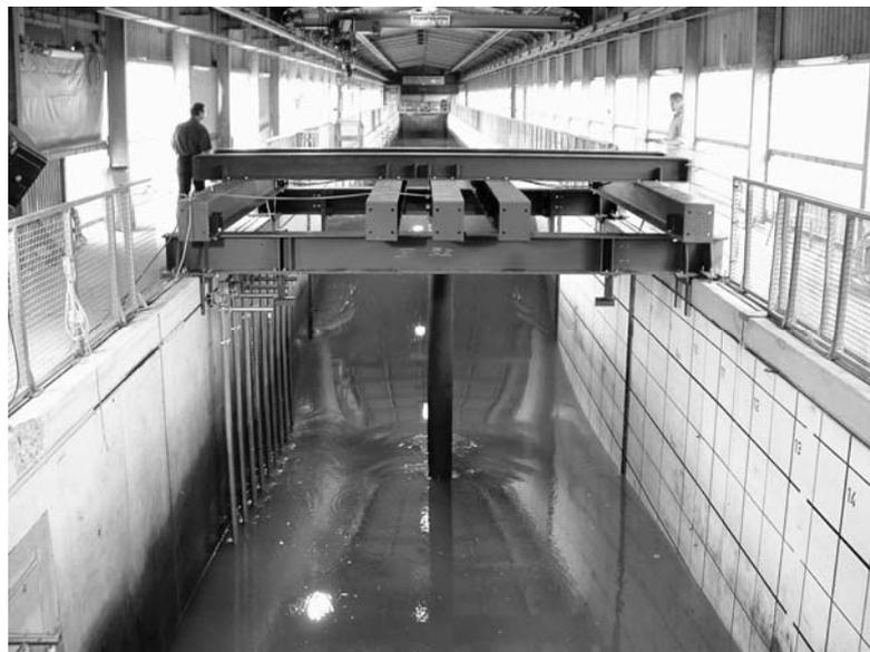
Figure 2. Model set-up with the measuring cylinder (Configuration 1, single isolated cylinder)
