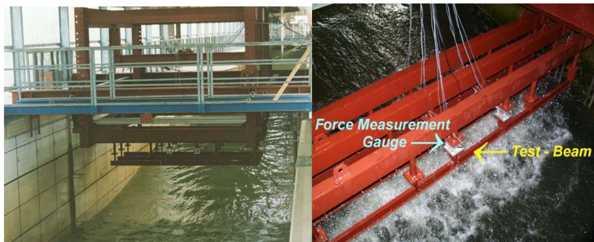
Figure 7-7. Support frame (left photo) and test with inundated element (right photo)
