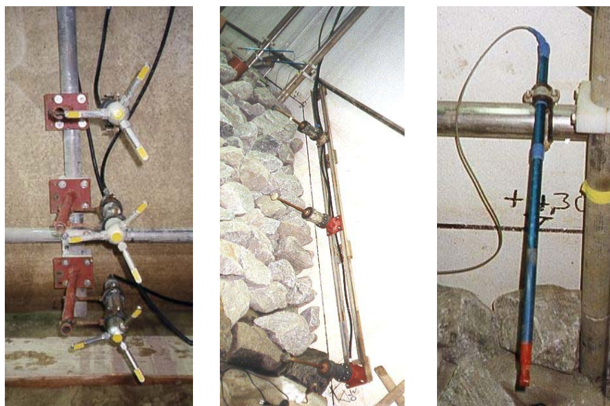
Figure 7-12. Orbital velocity component probes (Left: ADV-probes, middle: EMC - probes, right: Propeller probes)
