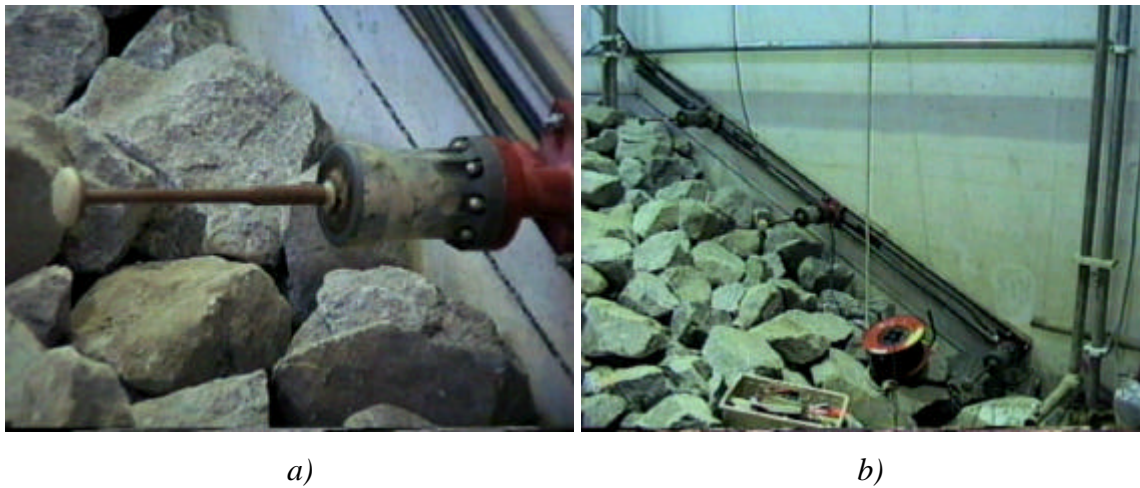
Fig. 8-6. ElectroMagnetic Current meters: a) instrument detail, b) 3 placed on the front slope
