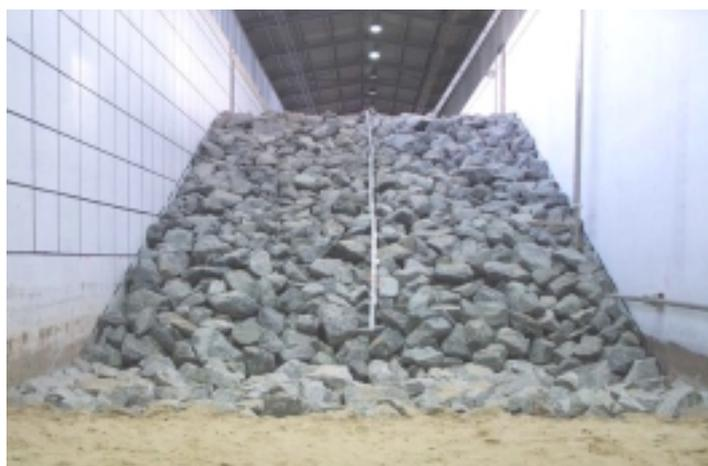
**Figure 4: View on the front slope of the breakwater with the run-up gauge.**
