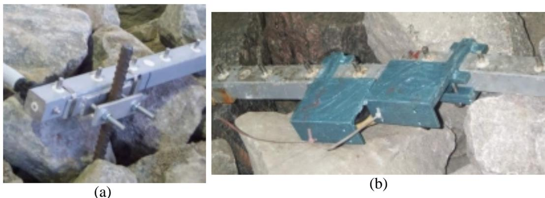
**Figure 5: (a) Clamps to fix the run-up gauges to steel bars driven into the core of the breakwater and (b) shield protecting the connection of the cables to the gauges.**
