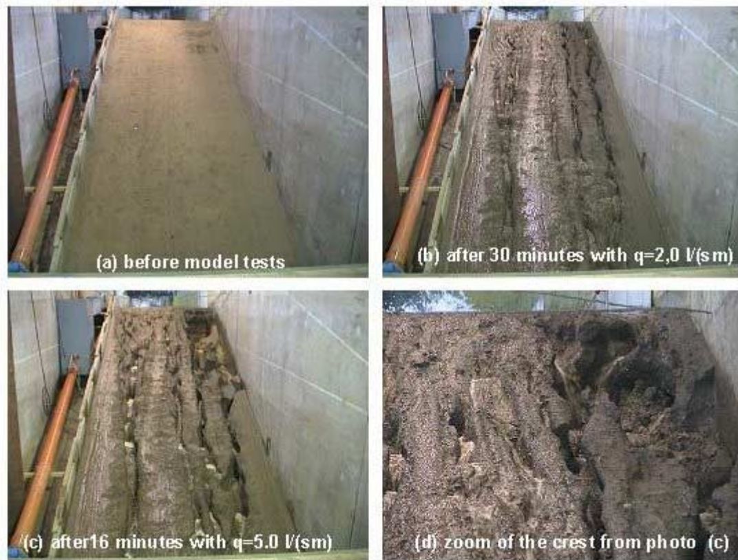
Fig. 12. Erosion Process during Model Test (Clay from Elisabethgroden km 3,5)
