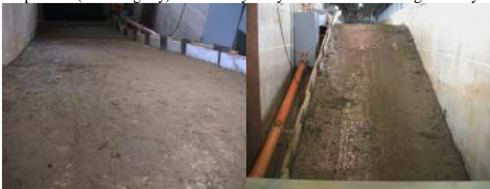
Fig. 9. Inner Slope before Model Testing (left) and Initiation of Erosion 2 Hours after Model Start (right) (Soil 1, q = 1.0 // (sm) )
