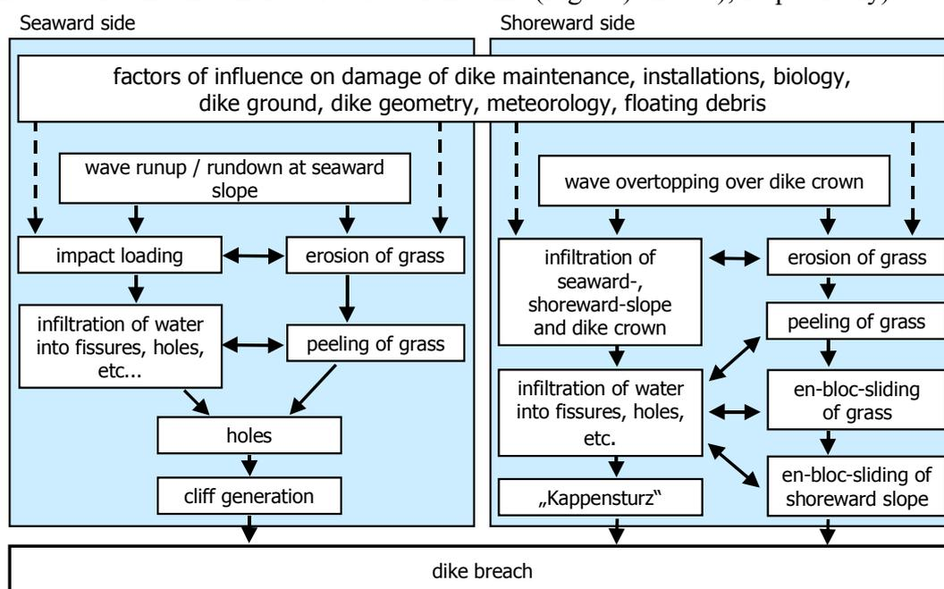
Fig. 4: Failure modes of seadikes eventually leading to dike breaching (a) seaward side, b) shoreward side)
