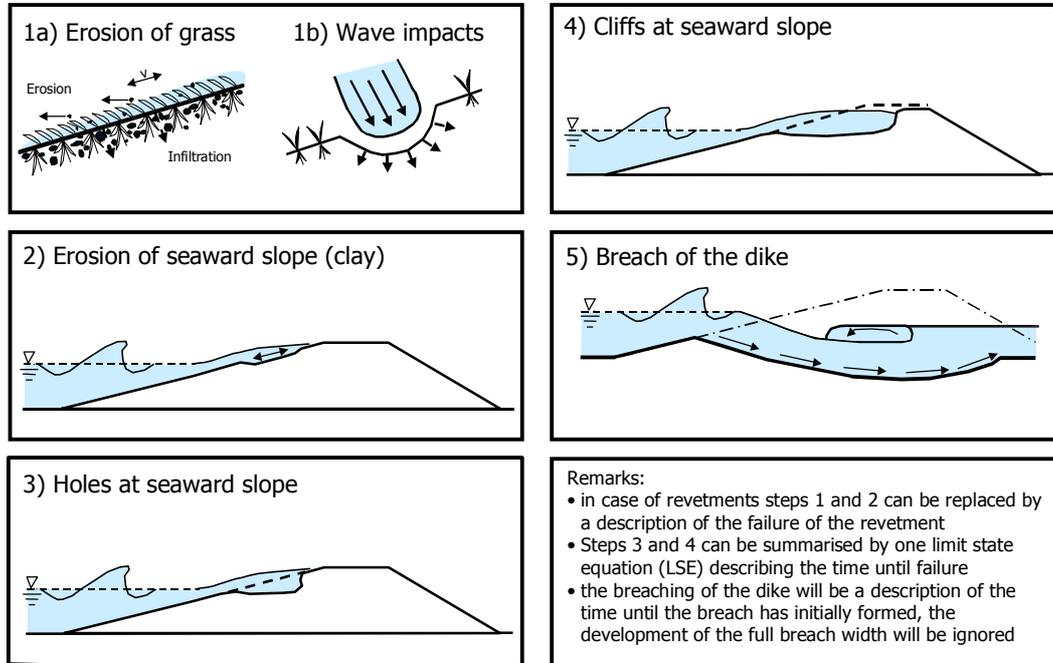
Fig. 5: Simplified description of processes at the seaward side of a seadike (after Oumeraci & Schüttrumpf, 1999)
