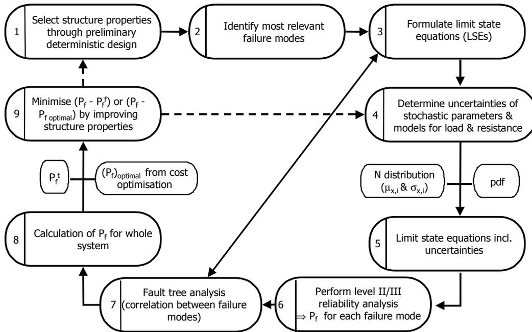
Fig. 2: Simplified flow chart illustrating the determination of a failure probability for a coastal defence structure
