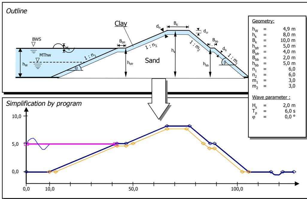
Fig. 7: Cross section and key parameters of an artificial example dike
