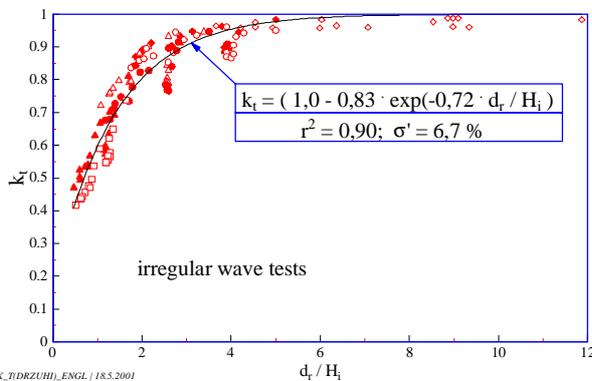
Fig.4: Relationship between transmission coefficient and dimensionless water depth
