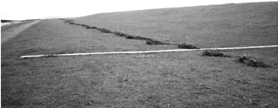
Fig. 1 Flotsam levels after a light storm surge event at one survey location
