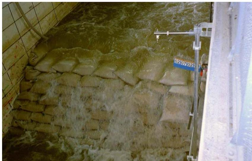
**Figure 11.** Sand container removed from structure slope
