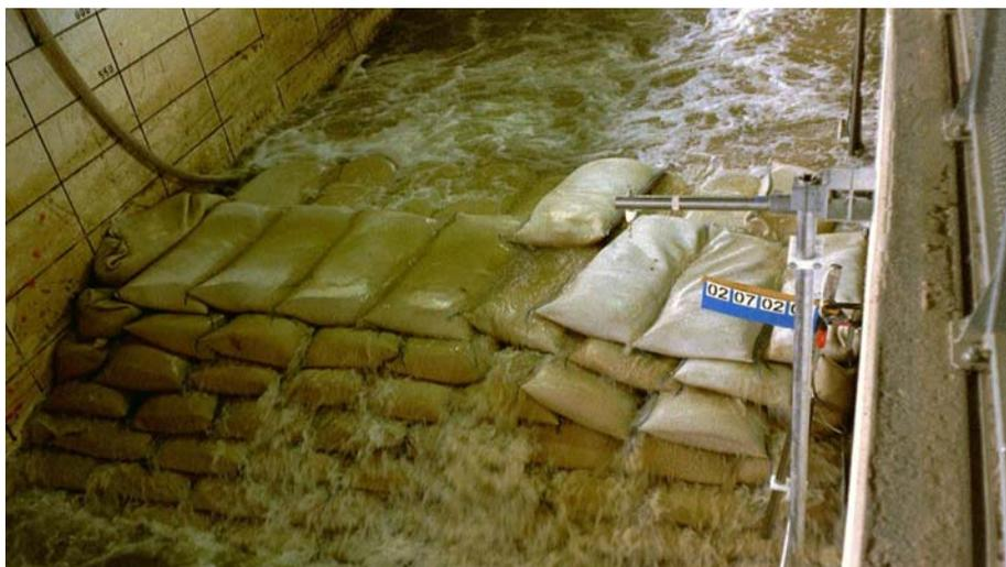
**Figure 13.** Sand container removed from crest of structure (GWK tests)
