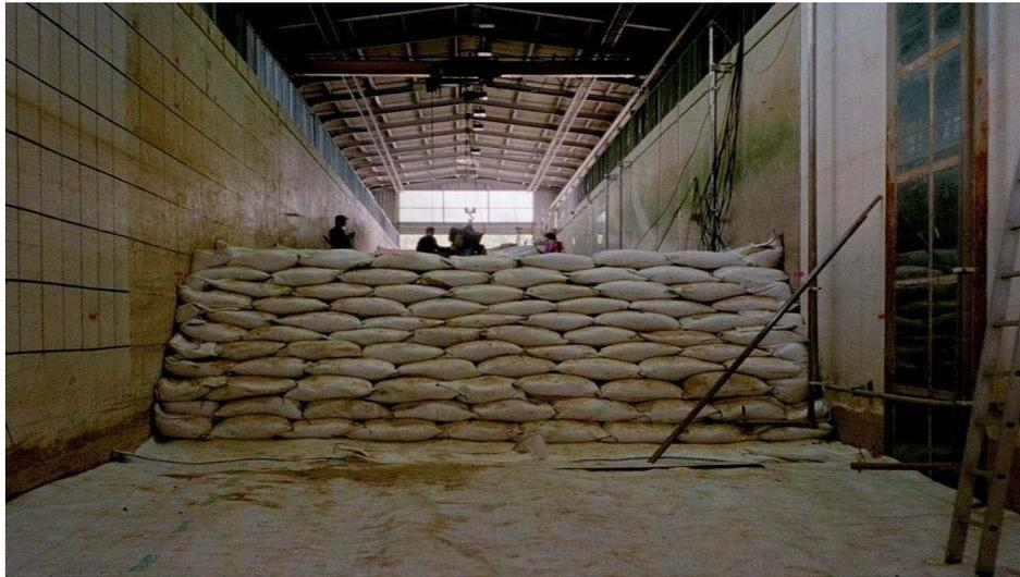
**Figure 6.** Large-scale model with 150 l sand containers in the Large Wave Flume of Hannover (GWK)
