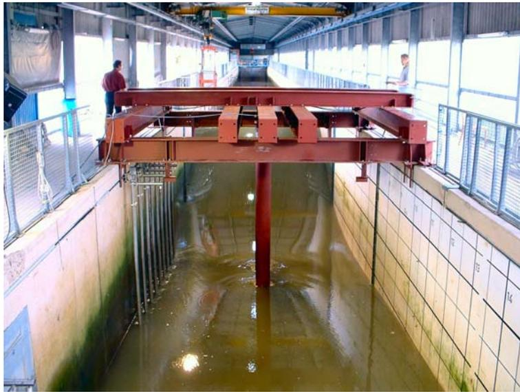
**Fig. 2. Model set-up with the measuring cylinder (configuration 1, single isolated cylinder)**
