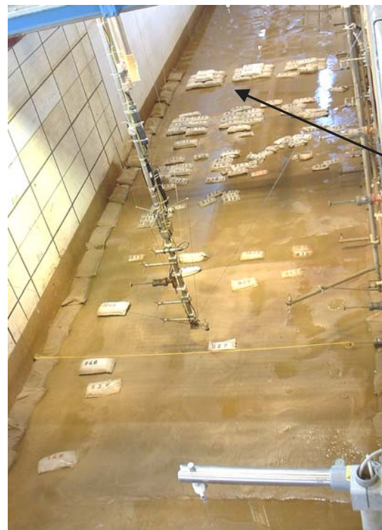
Displacements of sand containers after a test with H_{1/3} = 1.0 m, T_p = 5 s
