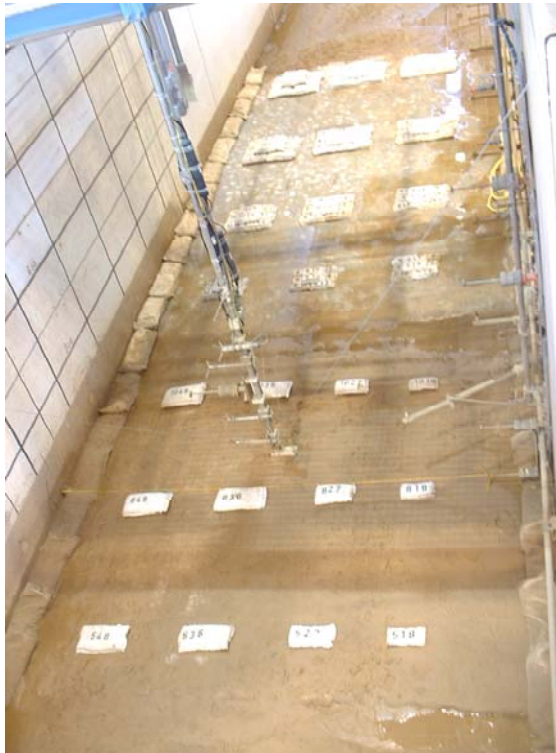
Sand containers placed transverse before tests
